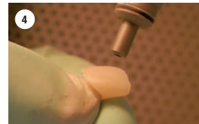
Perform Almina sandblast on the surface of the unpolished area of the crown (50~70µm, 30psi)
