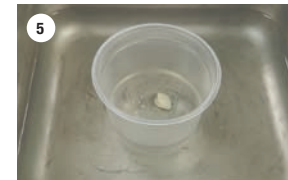
Clean restoration using an ultrasonic cleaner in alcohol or acetone, or steam cleaner
