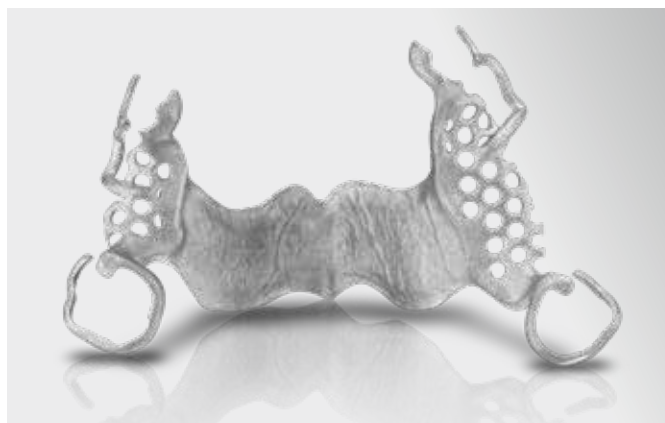
Partial denture from WIRONIUM® RP, sand-blasted
