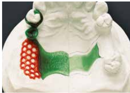
Coarsely grained casting wax on top of substructure made from smooth wax ensures defined plate thickness
