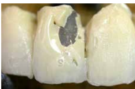
Bubbles and flaking/chipping
