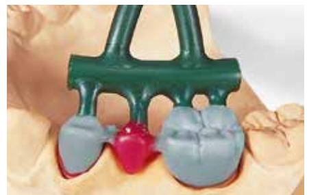
4 mm wax wire for feeding from the base socket mould former to the distribution channel
