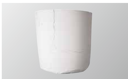
Mould with crack
