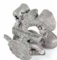
Rough casting due to overheating
