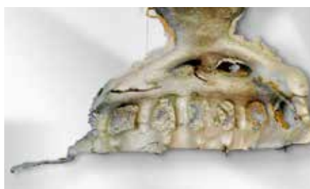
Casting flash on casting
