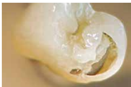
Bubbles in the ceramic
