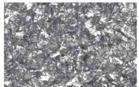
Wirobond® 280 blasted with Korox® 250 µm
