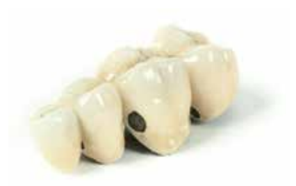
Bubbles in ceramic and insufficient ceramic bond to frame due to inadequate drying of paste opaquer
